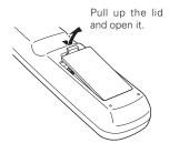
2 Install new batteries into the compartment.
