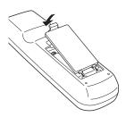
\* When the batteries of the remote control are replaced, the remote control code automatically returns to the initial code (Code 1) (p.41).
